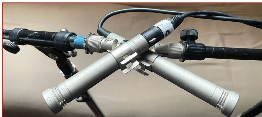
Two condenser microphones in an ORTF pattern.
