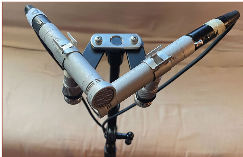
Two condenser microphones in an ORTF pattern.
