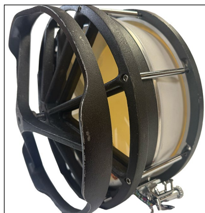
Bottom view of drum showing the 3-spoked base and internal 8-spoke frameworks that function as 1. the bottom rim and 2. control the rotary-tension process on the center, threaded bolt.
