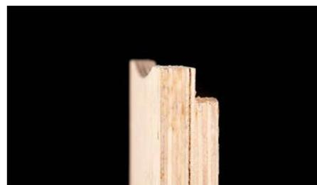
is up to six-inches long by 1/4-inch deep. The contour can be cut with a jig saw and further smoothed out with sandpaper. Image 9 shows the underside of the snare bed jig. A thin slot in the middle allows a small f-clamp to thread through the plywood in order to hold the shell firmly against the jig. The clamp can be adjusted by means of a channel which runs along the bottom of the jig as seen in Image 9. These elements of the jig can be cut with router bits of corresponding sizes.
