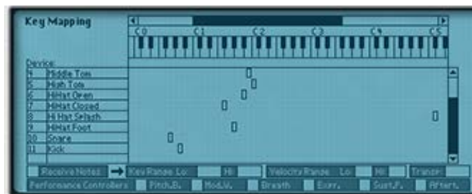
Figure 1: Individual MIDI notes received are mapped to different devices for each individual sound.
