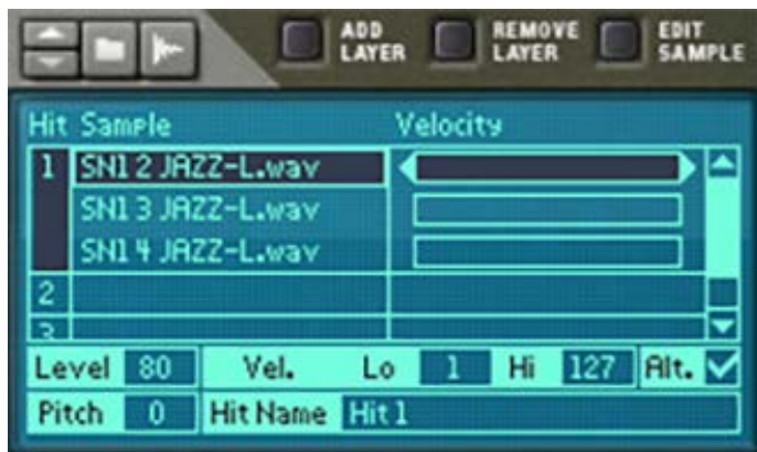
Figure 5: Three samples set to alternate randomly
