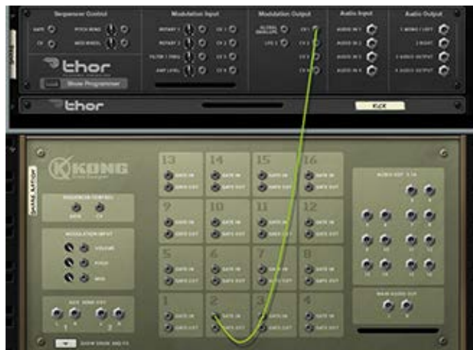
Figure 2: Mapping the snare drum MIDI to the snare drum pad on the Kong Drum Designer.
