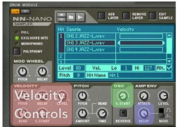
Figure 6: NN-Nano velocity controls highlighted in red, Sample Start highlighted in green, and decay highlighted in blue.
