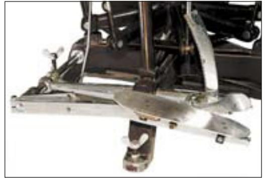
The clutch and ratchet tuning pedal, showing the lever arm attached to the side farthest from the player.
